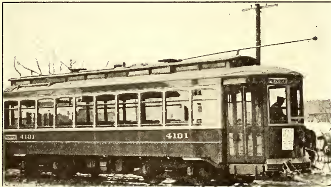
VIEW OF BAY STATE REMODELED CAR WITH INCLOSED VESTIBULES AND PNEUMATICALLY OPERATED DOORS AND STEPS
